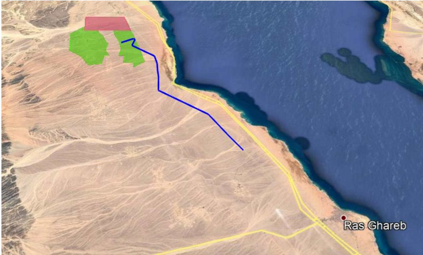
EETC Transmission line route to transfer electricity from the project substation to the national grid.
